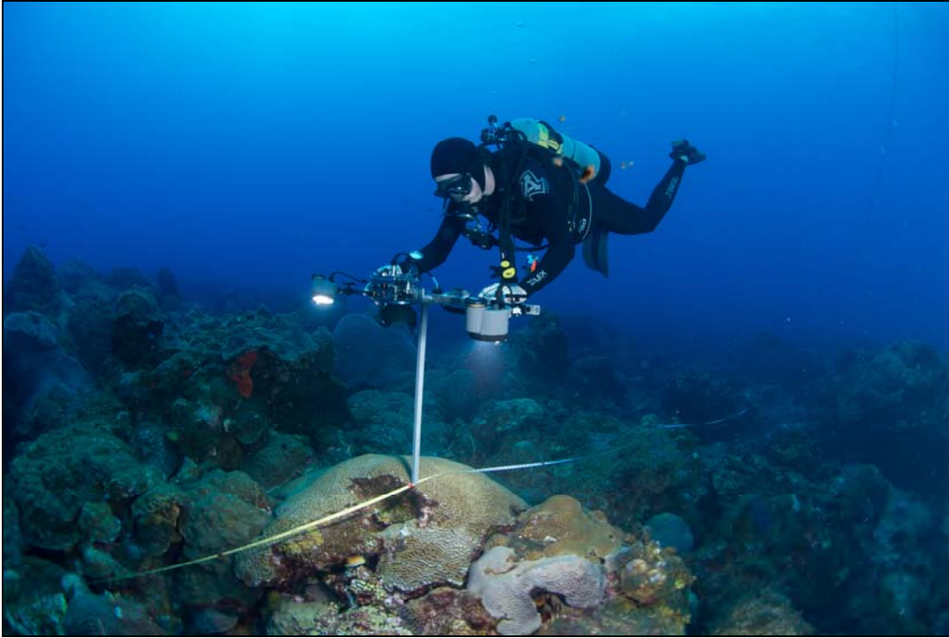
Figure 3.2.1. NOAA scientific diver with camera and strobes mounted on aluminum t-frame taking random transect photographs (NOAA/FGBNMS).
