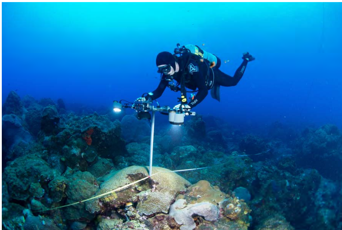
Figure 2.1. A camera and strobes are mounted on an aluminum t-frame to take random transect photos.
