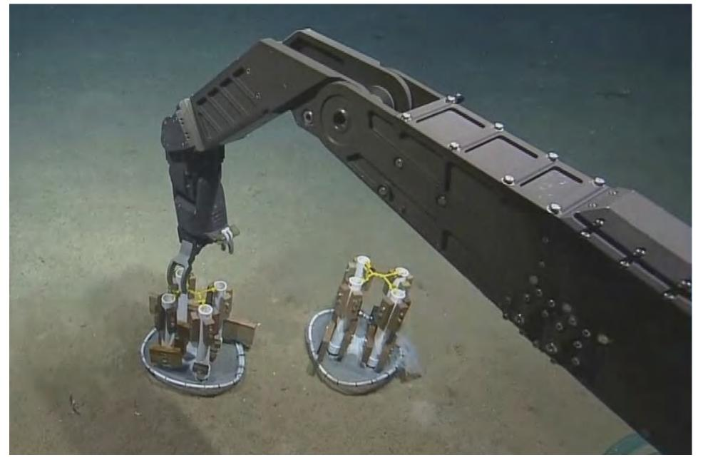
The manipulator arm of the remotely operated vehicle deploys two sets of wood experiments that are assessing the biological colonization and rates of degradation of wood used to build 19th century ships.
