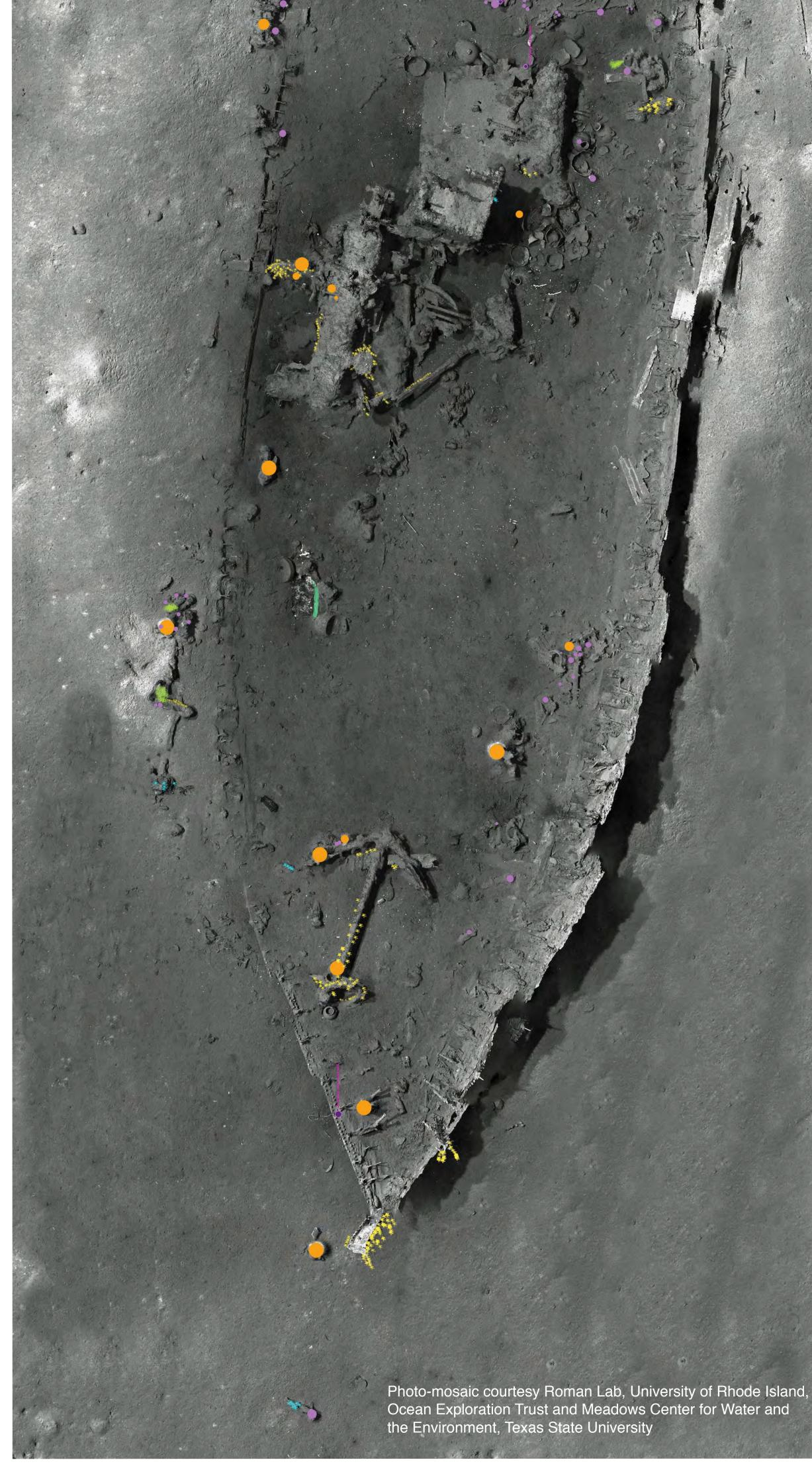
Wood degradation experiments have been deployed to evaluate the rate and processes of deterioration of different wood types at the wreck sites. Also, sediment core samples are being analyzed for benthic community structure and physiological processes influencing organic carbon and nitrogen content.
